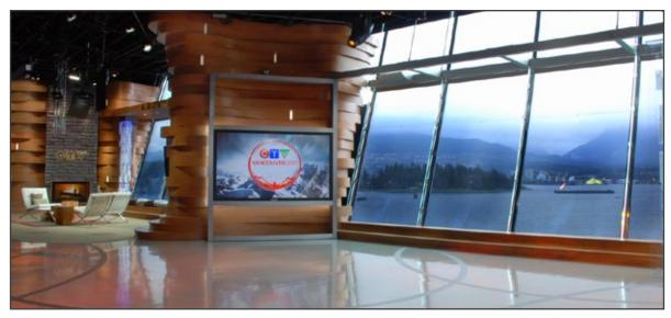
With RoscoVIEW panels on the windows, the exterior exposure can be easily controlled by rotating a matching camera filter.
