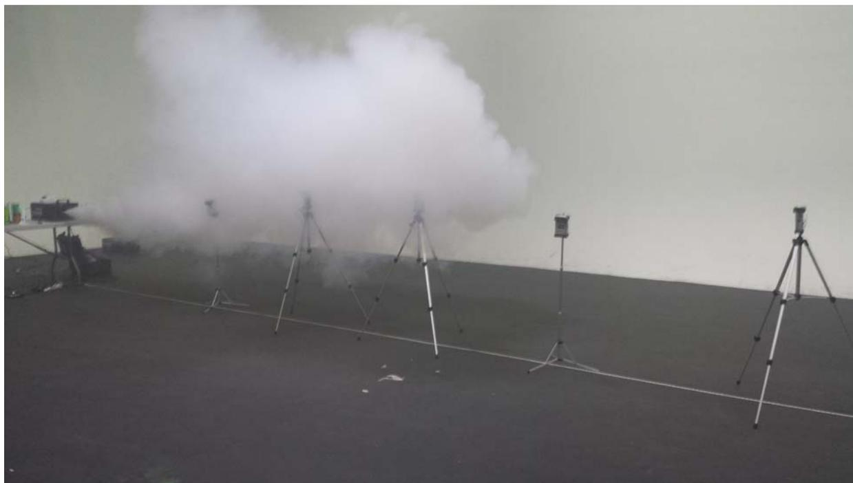
**Figure 2.** Monitoring configuration consisting of tripod mounted aerosol monitors situated at various intervals from the fog machine.
