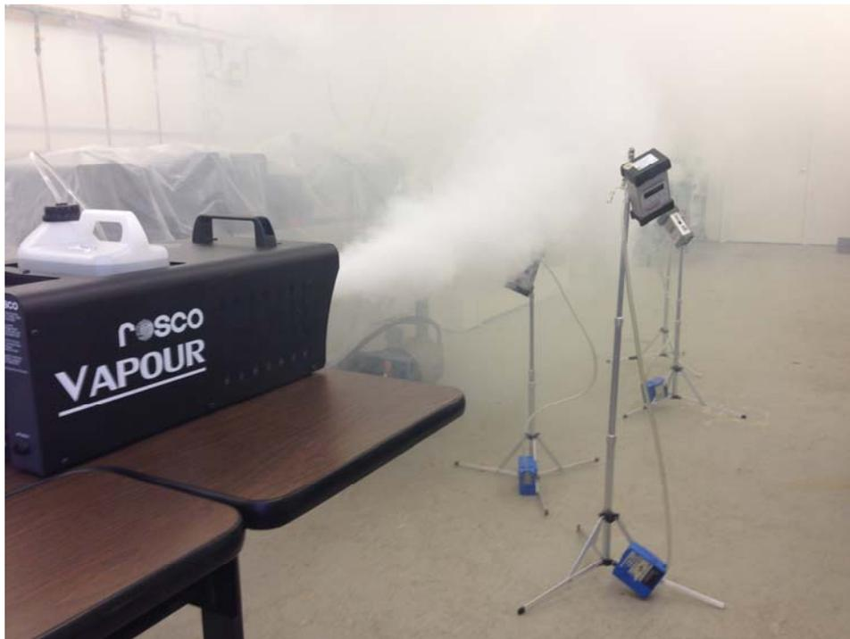
**Figure 1.** Configuration for calibration factor procedure, consisting of the tripod assemblies with sampling pumps, OVS tubes for sampling glycols, and aerosol monitors.
