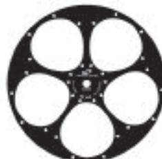
**Pattern 22: Colour Wheel** accepts five gels (held in place with standard paper fasteners) to give continual colour changes.
